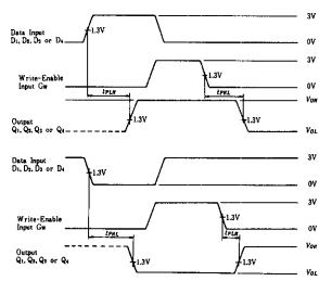
Each select address is tested. Prior to the start of each of the Note: above test both write and read address inputs are stabilized with  $W_A = R_A$  and  $W_B = R_B$ . During the test  $G_R$  is low.
