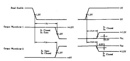
Waveform A is for an output with internal conditions such that the output is low except when disabled by the read-enable input. Waveform B is for an output with internal conditions such that the output is high except when disabled by the read-enable input.
